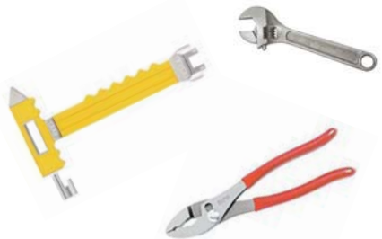
Tools to shut off utilities
